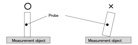
Press the probe quickly and smoothly to objects. A slow-acting press may cause large errors.
