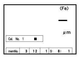
Measured data are stored in the following steps: Data are stored in order into a  $\lceil Group\ No. : 3 \rfloor$ ,
