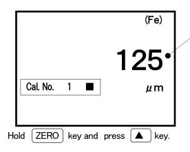
A measuring value is indicated and stored each time a probe is pressed in a normal state.
