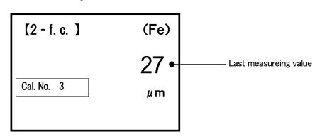
Equate this reading value with thickness Standard (in this example,  $25\,\mu$  m) by pressing  $\overline{\nabla}$  key.
