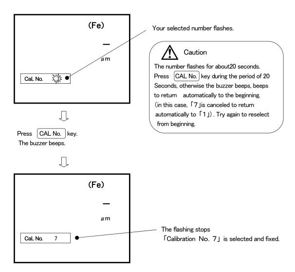
However, it may make errors depending on material formation and shapes to be measured. To minimize measurement errors and obtain as accurate results as possible please be sure of carrying out 2 kinds of adjustments of 「Zeroing」 and 「Calibration standard」 before measuring process.
