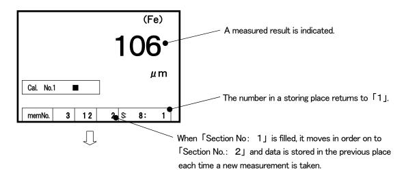
In a next case, As measurement data have been stored, they reached to a 「Section No.: 10」、a 「Data No.: 8」:
