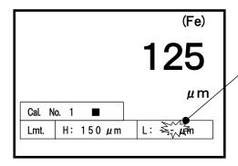
Press key to equate with necessary value. If the value exceeds the limit, press key, to decrease the value.
