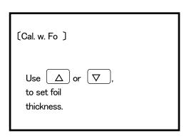
Equate a displayed value with Thic ness standard with key while the message is on the reading (20 seconds)
