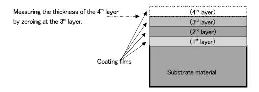
In case of being painted as shown with multi-layers on the substrate there may be needs to measure thicknesses of each layer. For example, measuring only the thickness of the 4<sup>th</sup> layer please zero as an assumed ZERO at the surface of the 3<sup>rd</sup> layer stacked on the substrate.
