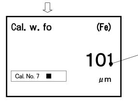
The last numerical v alue measured by probe
