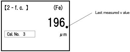
Equate the displayed value with the thickness of Thickness Standard (in this example 200  $\mu$  m) by pressing  $\blacktriangle$  key.
