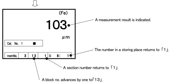
A storing place of  $\lceil B \mid B \mid B \rceil$  (  $= 8 \text{ data/section} \times 10 \text{ section} = 80 ) becomes full of measured data, and then accordingly in order moves forward to a <math>\lceil B \mid B \mid B \rceil$  each time measuring is taken.
