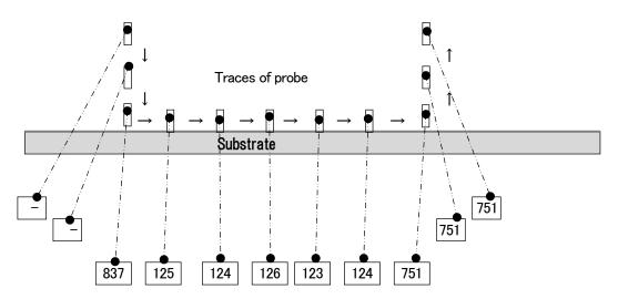
Measuring values on display (indicated with blinking successively each 0.5 seconds interval)
