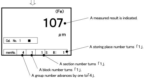
A storing place of 「Group No.: 3」 ( = 8 data/section × 10 section/block × 20 block = 1, 600 ) becomes full of measured data, and then accordingly in order moves forward 「Group No.: 4」 each time a measurement is taken.
