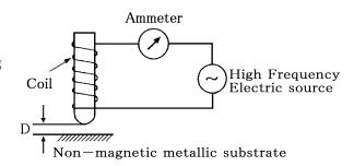
by a high frequency electric source, the current increases or decreases in accordance with a distance from the coil.
