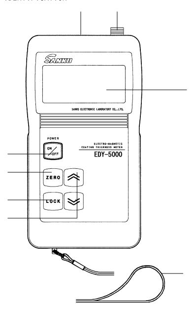
POWER key Key for power ON/OFF ZERO key Key for zero adjustment
